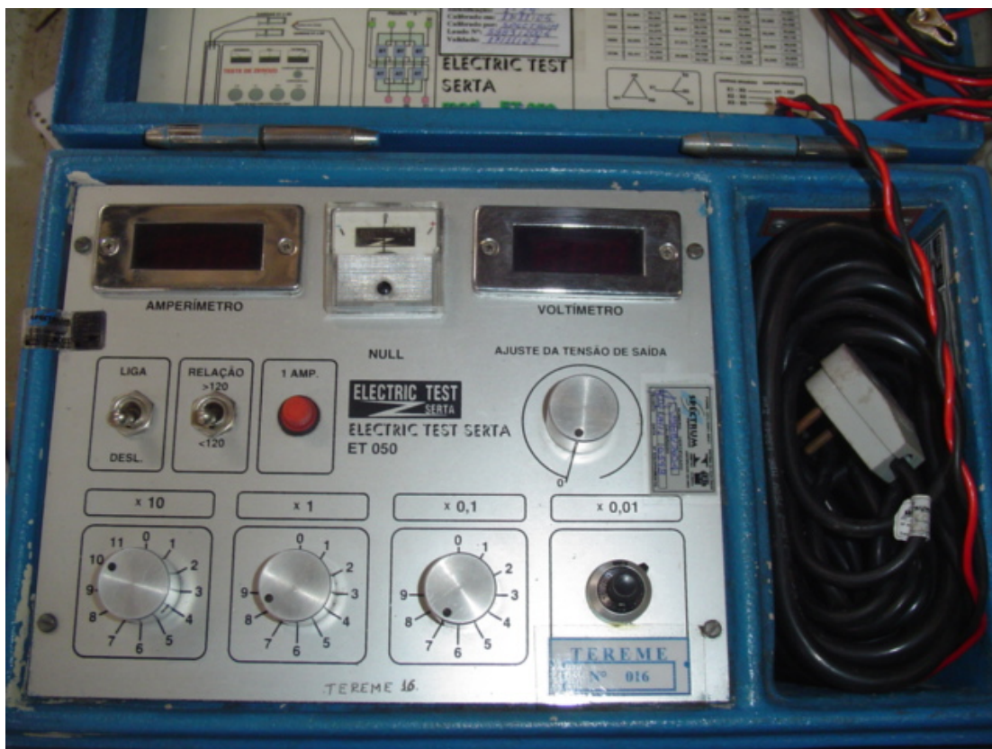
Fig 39 TTR (Transformer Turn Ratio)
